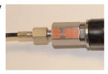
5) When charging is complete, "bleed" off the excess air from the hose using the hoses's bleed screw. Then unscrew the bottle from the charging adaptor.
